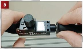
Hold both probe and sensor simultaneously when inserting the rubber sleeve to avoid damaging the two optical fibres on the level of the rivets.
