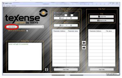
Once the search is done the list next to the search button should contain all the texense sensors detected on the CAN bus (1). Select the sensor you want to configure and click on the button in the read panel (2) to display sensor's configuration:
