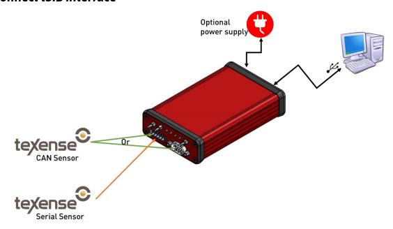
Connect the tSIB to the computer using the USB-A to USB-C cable provided. Power LED of the tSIB should be on.
